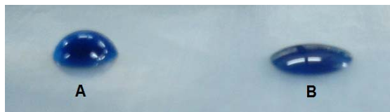
Figure 1. Drop collapse assay. Collapsed droplets (A) is H 2 O and (B) is Lactobacillus acidophilus ATCC 4356-derived biosurfactant
