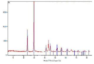
Figure 2. X-ray diffraction patterns of Se-nanoparticles. The highest peak is recorded in 29.73 and 23.523 (°2Th) positions
