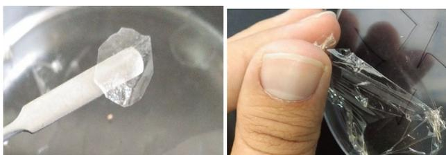
**Figure 6.** ALG-L12-LNZ insert, film formation (left), film separation (right)
