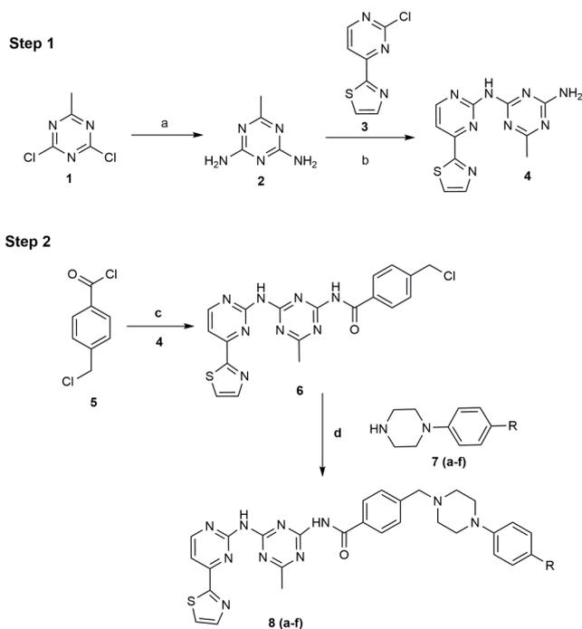
**Scheme 1.** Reagents and conditions: a) Liq. NH<sub>3</sub>, 40-45 °C, NaHCO<sub>3</sub>, heat, 2-3 hr, b) NaOBu-t/THF 10 °C to RT, 2 hr, c) THF-TEA, 0 °C, 3 hr, d) reflux, 3-5 hr
