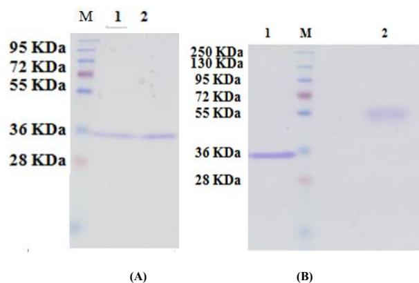
**Figure 9.** After dialyzing, wild-type and mutant recombinant streptavidin were analyzed on SDS-PAGE gel in the presence and absence of biotin. A: M, protein marker. Lane 1 and 2: mutant recombinant streptavidin in the presence and absence of biotin. B: M, protein marker. Lane 1: Recombinant streptavidin in absence of biotin. Lane 2: wt recombinant streptavidin in the presence of biotin
