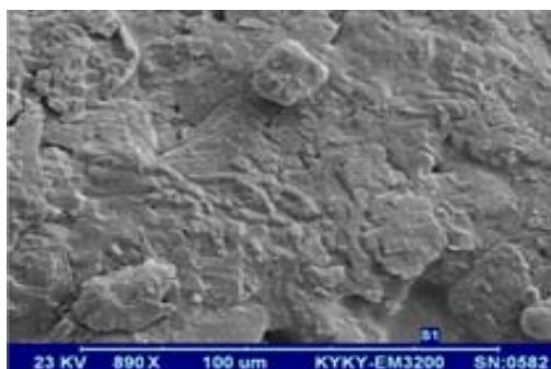
**Figure 2a.** SEM of pellets containing 20% plasticizer, cured at 40 °C for 24 hr with a magnification 890 × ( $S_1$ )
