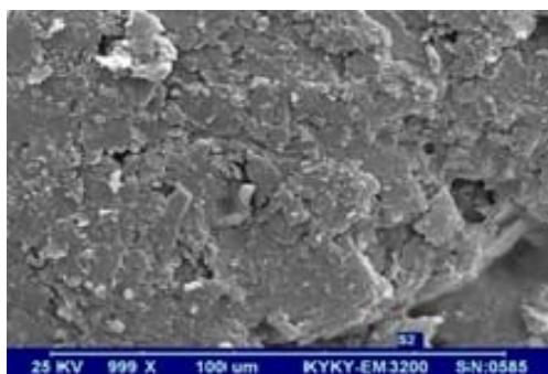
**Figure 2b.** SEM of pellets containing 20% plasticizer, cured at 60 °C for 168 rh with a magnification 999 × ( $S_2$ )
