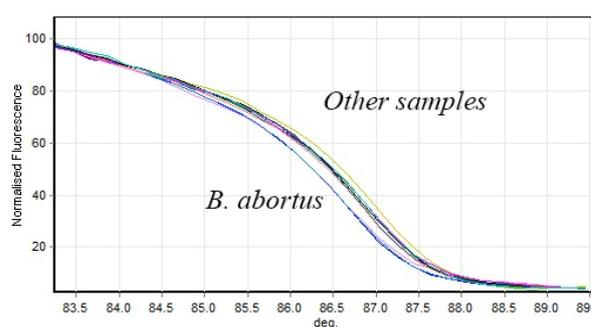
**Figure 4.** HRM assay separation curve of *Brucella abortus* from other species. *glk* target gene was amplified for the *Brucella* species using the special primer with 164 bps. Data shows the analysis of high-resolution melt curve for separation of *B. abortus* with mutation of guanine in 164 bps from *glk* gene
