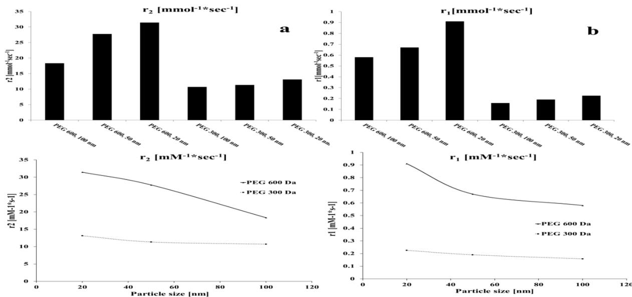
Figure 3. Plots of (a)  $r_2$  and (b)  $r_1$  relaxivity versus particle size of PEGylated iron oxide nanoparticles
