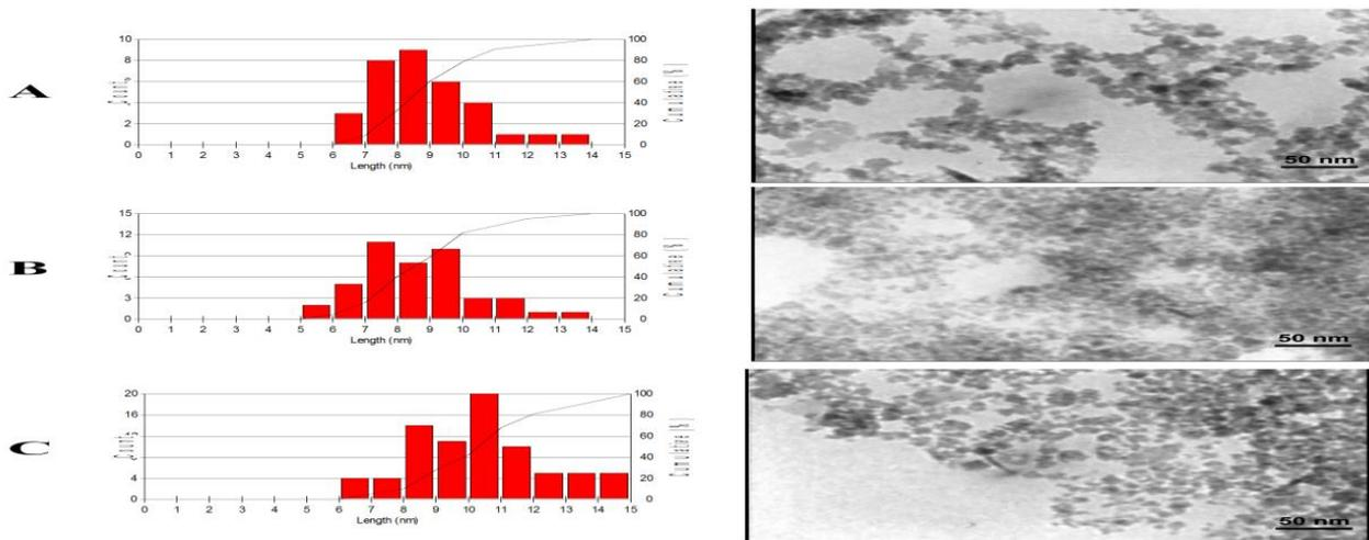
Figure 1. TEM image and histogram of PEGylated iron oxide nanoparticles. A. 20 nm, B. 50 nm and C. 100 nm.
