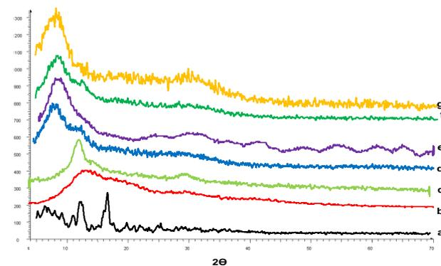
**Figure 5.** XRD thermogram of Ketotifen fumarate (a); Eudragit RL 100 (b); PVA (c); blank NPs of F<sub>2</sub> (d); F<sub>1</sub> (e); F<sub>2</sub> (f); F<sub>3</sub> (g), respectively
