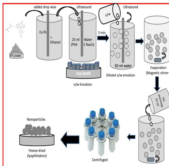
**Figure 1.** Nanoparticles preparation procedure with Eudragit RL 100 polymer
