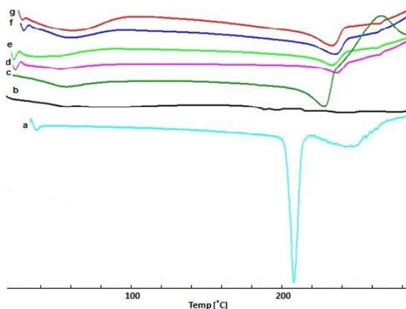
**Figure 4.** DSC thermogram of Ketotifen fumarate (a); Eudragit RL 100 (b); PVA (c); blank NPs of F<sub>2</sub> (d); F<sub>1</sub> (KF:EU) 1:7.5 ratio (e); F<sub>2</sub> (KF:EU) 1:10 ratio (f); F<sub>3</sub> (KF:EU) 1:10 ratio (g), respectively
