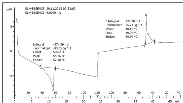
**Figure 5.** Differential scanning calorimetry (DSC) thermogram of *Z. multiflora* essential oil-loaded solid lipid nanoparticles prepared by 5 cycles of high shear homogenization and ultra sound technique. 5 mg of sample was used in each run
