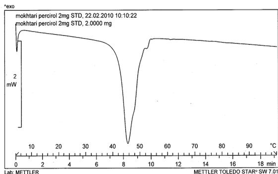
**Figure 3.** Differential scanning calorimetry (DSC) thermogram of Precirol ATO5 5mg of lyophilized powder was used in each run
