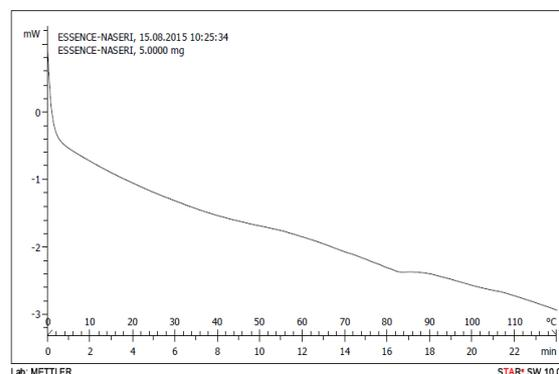
**Figure 2.** Differential scanning calorimetry (DSC) thermogram of *Z. multiflora* essential oil prepared by high shear homogenization and ultra sound technique. 5 mg of sample was used in each run
