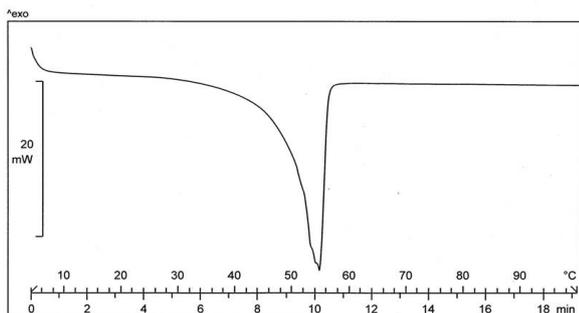
**Figure 4.** Differential scanning calorimetry (DSC) thermogram of Glyceryl mono stearate (GMS) 5mg of lyophilized powder was used in each run
