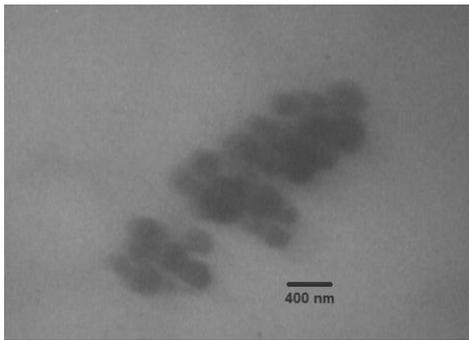
**Figure 1.** A transmission electron microscopy (TEM) image of Interleukin-12 loaded chitosan nanoparticles
