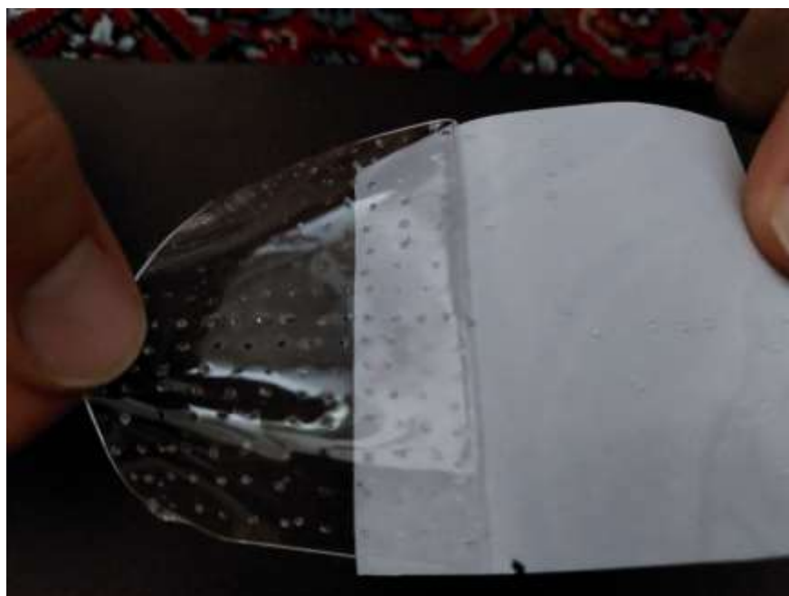
Figure 4. The silicone layer separation from greaseproof paper
