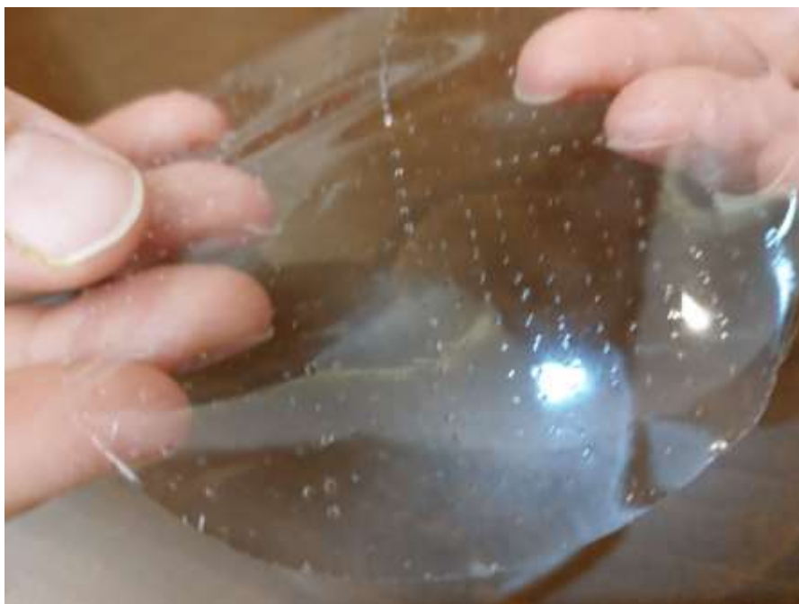
Figure 3. The 1 mm silicone layer after punching
