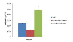
**Figure 3.** The density of attached H9C2 cells to tissue culture polystyrene (n=18), unanodized (n=3) and anodized titanium with nanotube structures (n=21). Cell adhesion was evaluated by counting stained nuclei of attached cell/cm² of substance surface. \* denotes P<0.05. Data are expressed as mean±SEM
