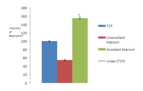
**Figure 2.** Cell survival and proliferation on tissue culture polystyrene, unanodized titanium and anodized titanium with nanotube structures (%). Cell survival and proliferation were evaluated using MTT test. \* denotes P<0.05. Data are expressed as mean $\pm$ SEM (n=3)
