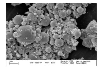
Figure 3. Scanning electron micrograph of alginate microspheres (B-5 batch).
