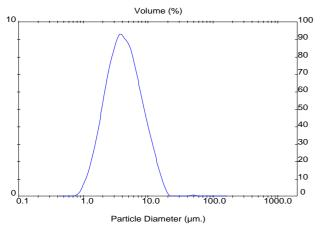
Figure 2. Size distribution curve of B-5 batch. Particle size (volume mean diameter) and size distribution of the microspheres of the batch-6 was determined using a particle size analyzer.
