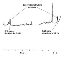
Figure 5. The expanded <sup>1</sup>H-NMR spectrum of *A. annua* extract with protons B (methylene protons) signals appeared at 5.46 and 6.18 ppm as doublets.
