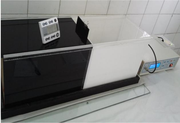
**Figure 2.** Passive-avoidance apparatus (step-through type)
